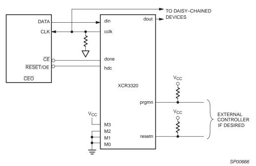
Figure 17: Master Serial Configuration
