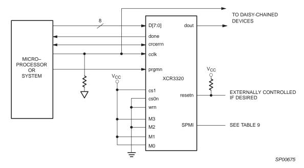
Figure 21: Synchronous Peripheral Configuration
