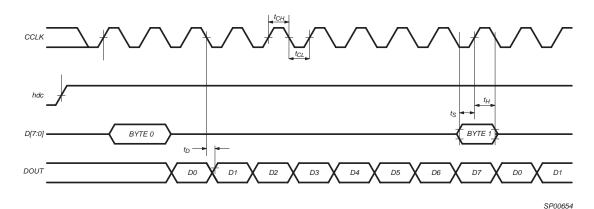
Figure 26: Slave Parallel Configuration Mode Timing Diagram
