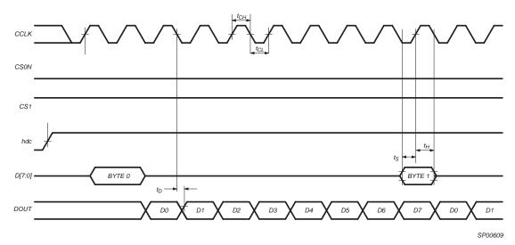
Figure 22: Synchronous Peripheral Configuration Mode Timing Diagram
