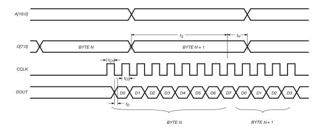
Figure 20: Master Parallel Configuration Mode Timing Diagram
