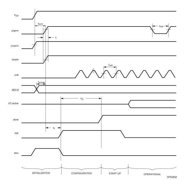
Figure 9: General Configuration Mode Timing Diagram
