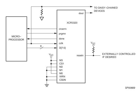
Figure 25: Slave Parallel Configuration Schematic
