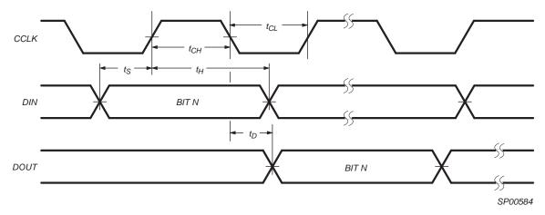
Figure 18: Master Serial Configuration Mode Timing Diagram
