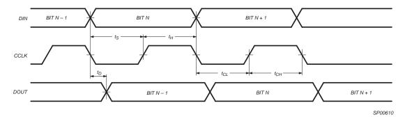
Figure 24: Slave Serial Configuration Mode Timing Diagram
