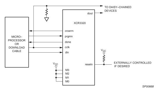
Figure 23: Slave Serial Configuration Schematic
