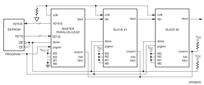
Figure 27: Daisy-Chain Schematic with Lead Device in Master Parallel
