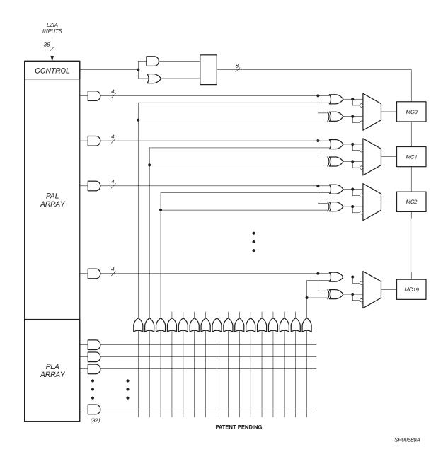
Figure 3: Xilinx XPLA2 Logic Block Architecture
