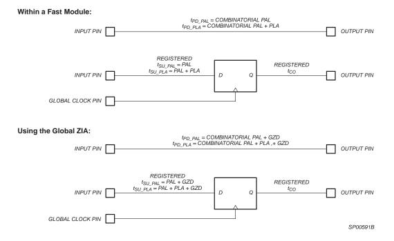
Figure 5: XCR3320 Timing Module
