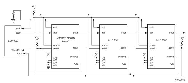
Figure 28: Daisy Chain Schematic with Master Serial Lead Device
