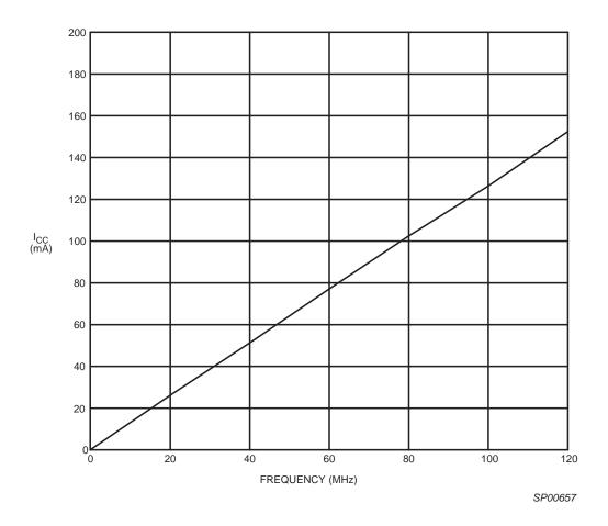
Figure 6: I<sub>CC</sub> vs. Frequency at V<sub>CC</sub> = 3.3V, 25°C
