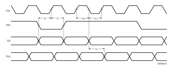
Figure 29: Boundary Scan Timing Diagram
